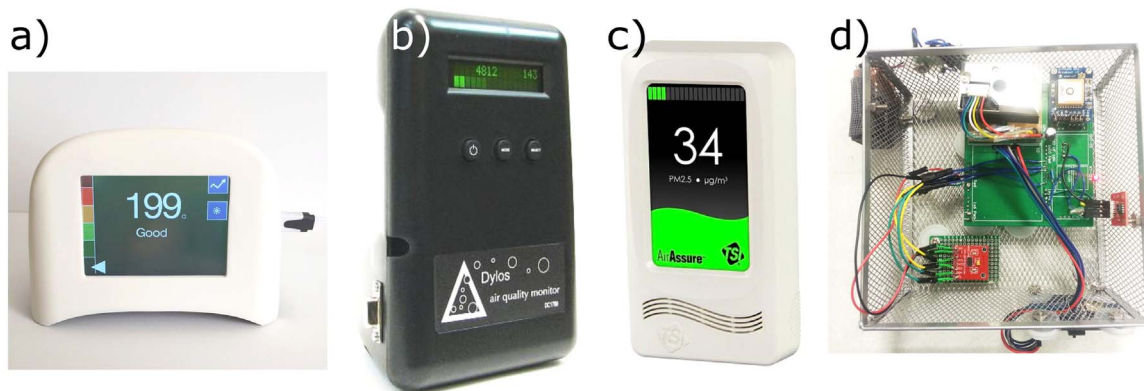
Fig. 1. Monitors used in this study: (a) Speck ( https://www.specksensor.com/ ), (b) Dylos 1700 ( http://www.dyloproducts.com/ ), (c) TSI AirAssure ( http://www.tsi.com/airassure-pm2-5-indoor-air-quality-monitor-en/ ), and (d) UBAS (photo taken from a manual).
